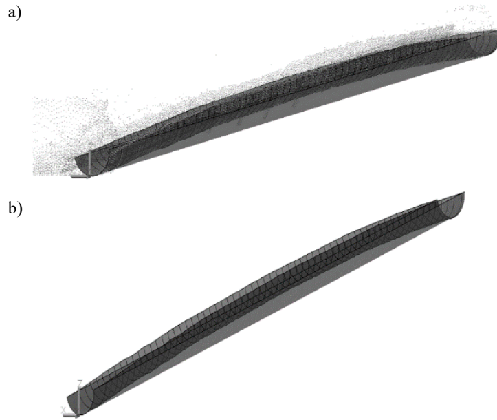
Fig. 3. Deformation of the gutter – reference and real models: a) on the point cloud background, b) without the point cloud ( own research )
