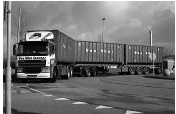
Figure 5. Short three container B-Triple (the Netherlands).
