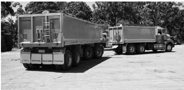
Figure 7. PBS Rigid truck and 4 axle trailer (Australia) Source Industrial Logistics Institute database.
