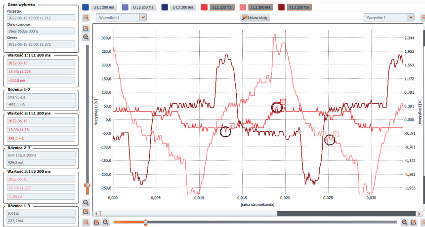
Fig. 5. Current waveforms recorded for electrical installation at idle*
