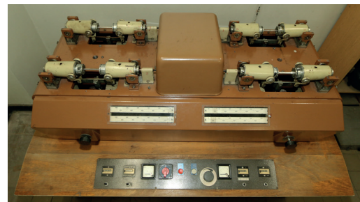
Fig. 1. Machine for high-cycle fatigue testing under conditions of rotary bending
