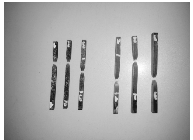
Figure 11. The specimens after completion the tensile test
