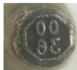
Fig. 9. Marker with WC-Co electro-spark coating
