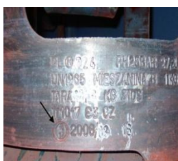
Fig. 7. The flange of a gas cylinder with a permanent mark
