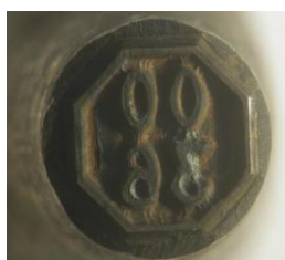
Fig. 8. Worn marker intended for regeneration
