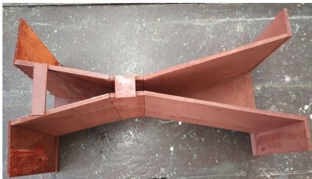
Fig. 3. View of a Parshall flume model
