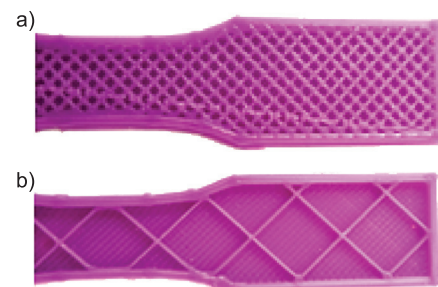
Fig. 4. Shoulder segment of tensile test specimens with a print density of 50% (a) and 10% (b) made of PLA
