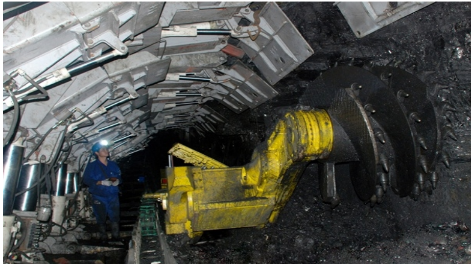
Fig. 1. A long-wall cutter in the Halam mine in Halong.
