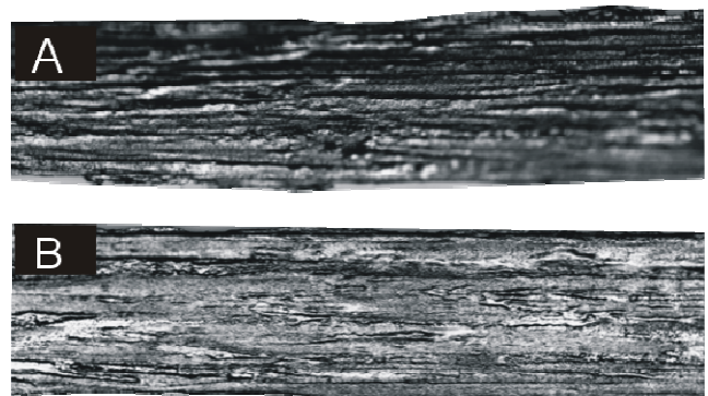
Fig. 9. View of the ribbon surface: A – atmosphere side; B – Cu wheel side
