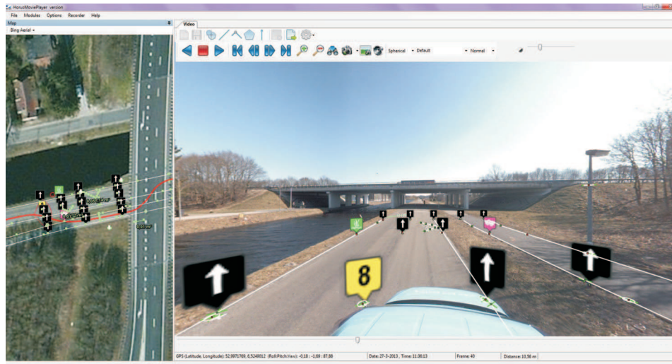
Fig. 6. The drive through a road with multiple annotations. These arrows (icons) contain information which can be accessed interactively and are changing their position on the displayed geo-referenced panoramic videography. Permission to reproduce this image has been granted by Dirk Aalbers
