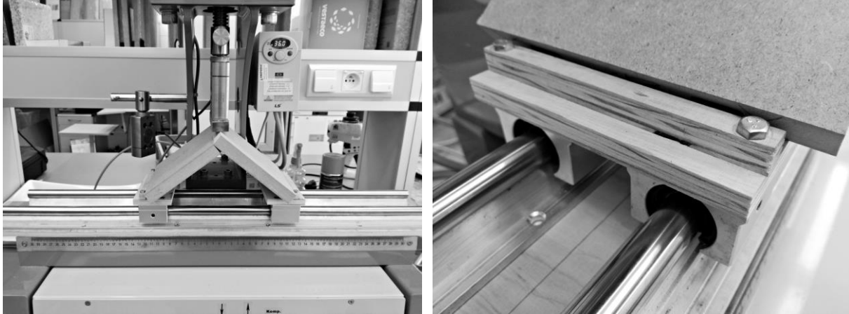
Fig. 3. The test stand with the use of a special equipment for fixing the samples on the testing machine
