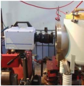
Fig. 6. Test stand with a dismantlable vacuum chamber and a high speed camera
