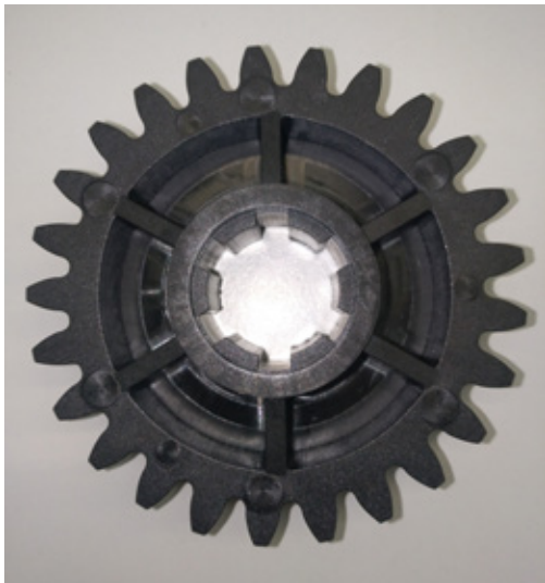
Fig. 6. Injection mold seat for the KZ25 gear wheel
