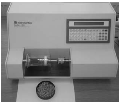
Fig. 2. Envelope Density Analyzer GeoPyc 1360
