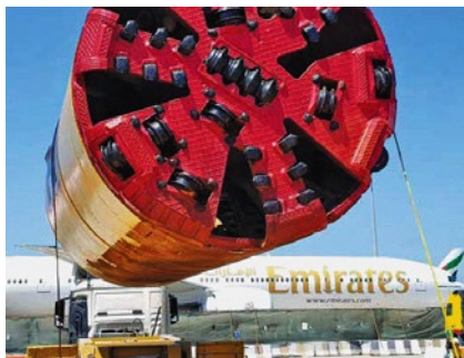
Ryc. 4. Maszyna AVND2400AB MTBM firmy Herrenknecht [2]
