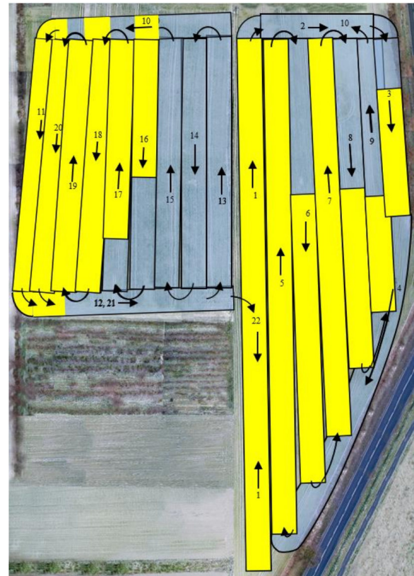
Fig. 16. Orthophotos with marked tracks for agricultural aeral requiring fertilization
