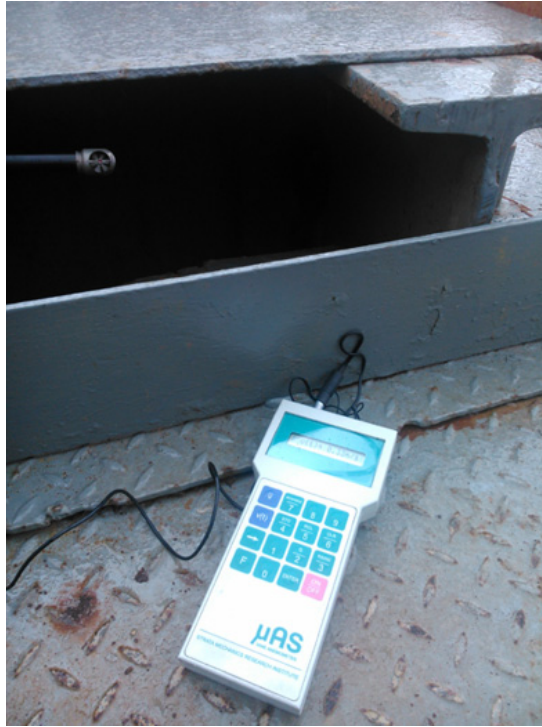
Fig. 4. Air velocity measurements at point no. 2
