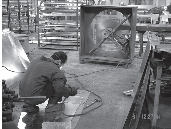
Figure 4. Worksite before improvement: no cover on fan, poor posture due to lack of table.
