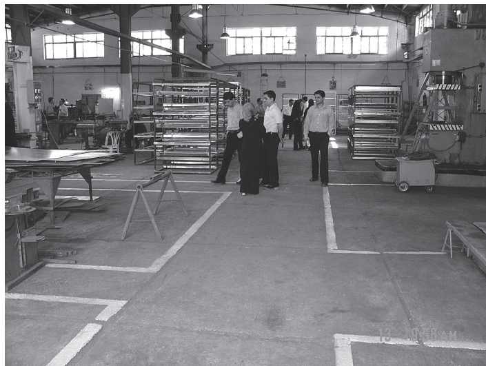
Figure 6. Worksite after improvement: lines separate transport areas from working areas, transport areas clear.
