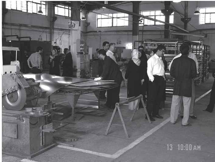
Figure 7. Worksite after improvement: a working table for laminator, though its height is not suitable yet.
