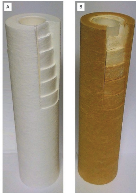
Fig. 6. Filter for testing; A – clean filter, B – filter loaded with solid contamination
