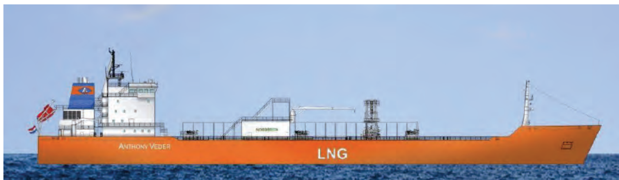
Fig. 6. 15600 m 3 LNG carrier (TGE-Marine design) – delivered December 2012 [13]
