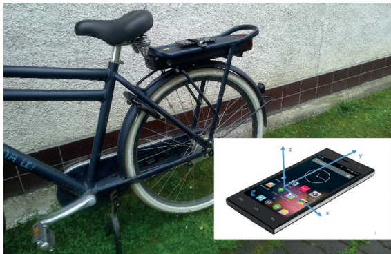
Fig. 2. Instrumental bicycle and smartphone indicating the x, y, z axes of the accelerometer
