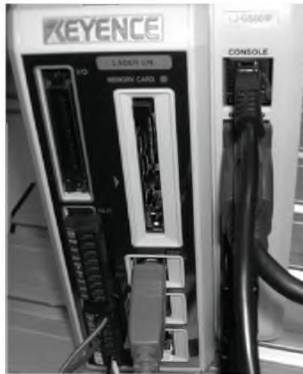
Fig. 8. Scanning head LJ-G50001P controller
