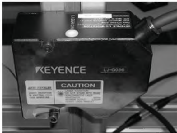
Fig. 6. Exemplary view of the Keyence LJ-G030 laser scanning head used for the Project
