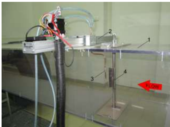
Fig. 3. A crucial part of stand for flowmeter tests: 1-measurement part of wind tunnel, 2-linear module with stepper motor, 3- two-directional probe, 4-tested two-profile probe
