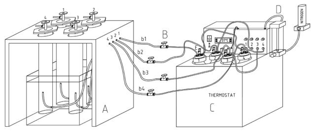
**Figure 2** Quadruplicate bioreactor set for dark fermentation of differentiated broths combined with gas accretion volume measurement (A – gas accretion measuring system, B – tree-way valve, C – thermostat, D – nitrogen line, E – bioreactors 4 × 50 mL)
