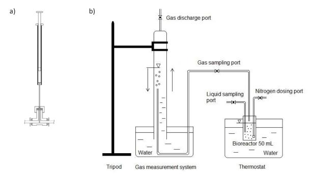
Figure 3 a) A three-way valve and a gas tight syringe for gas sampling during dark fermentation, b) Schematic diagram of a single bioreactor and gas collecting system connection
