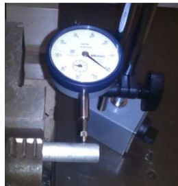
Fig. 16. Runout measurement using a dial indicator.
