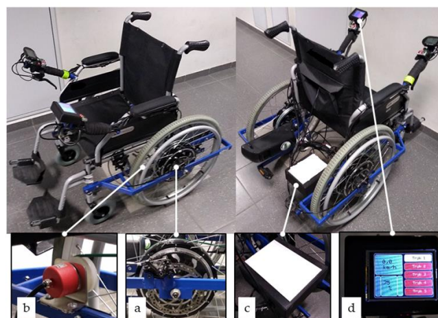
Fig. 2. The tested AR-405 wheelchair is equipped with a hybrid propulsion module. a – power of 500 W installed in the drive wheel hubs; b – incremental encoders; c – proprietary control system with a gyroscope; d – touch screen controller
