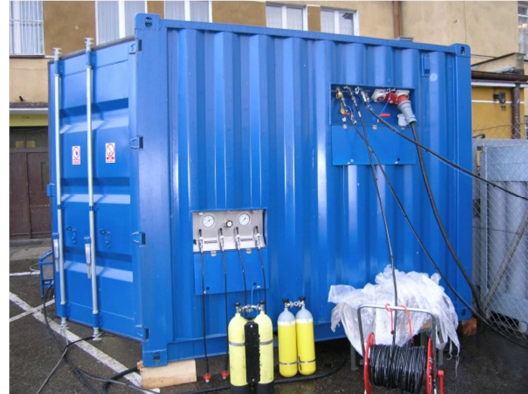
Fig. 21 General view of the Mobile Air Supply Set container. Source: own study.
