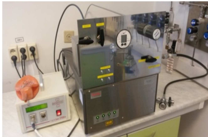
Fig. 3-4 FTIR Spectrometer NICOLET ANTARIS Thermo Scientific with zirconium oxygen analyser RAPIDOX 2100ZF.
