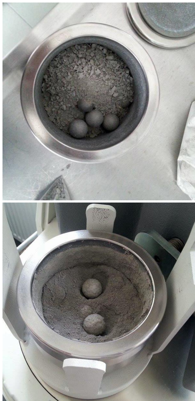
Fig. 1. Material for the recycled binder powder during milling.
