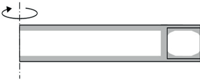
Fig. 4. Stage II – closure of air bubble
