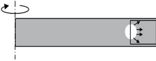
Fig. 7 Stage IV – pushing the bubble out of the preform; ← indicates the direction of capillary pressure
