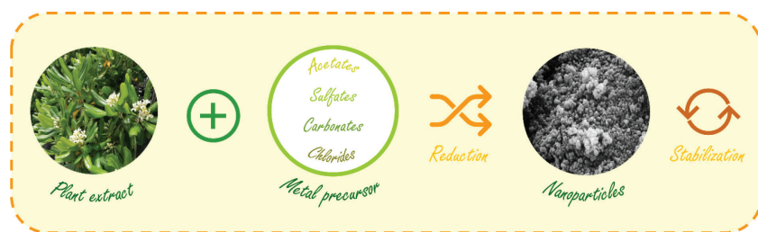
Fig. 3. The scheme for the green synthesis of metallic NPs with the use of plant extract
