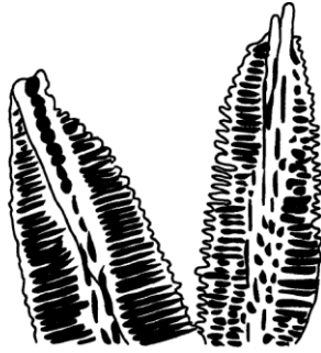
Fig. 3. Model of the structure of ledeburite growth by Rickard and Hughes [4]
