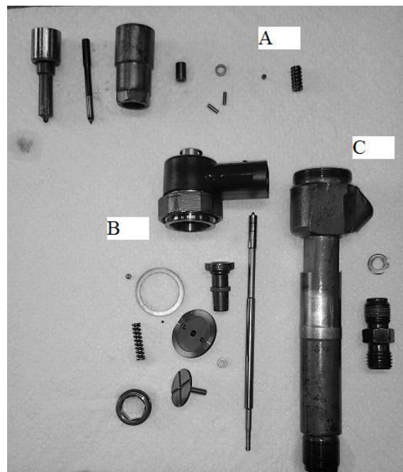
Fig. 2. Common Rail fuel injector disassembled into spare parts: A – atomizer part, B – steering part, C – main body part
