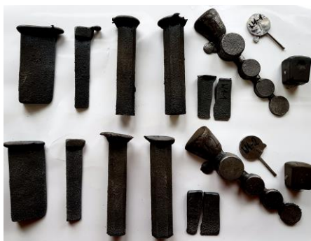
Fig. 8. A set of cast test specimens
