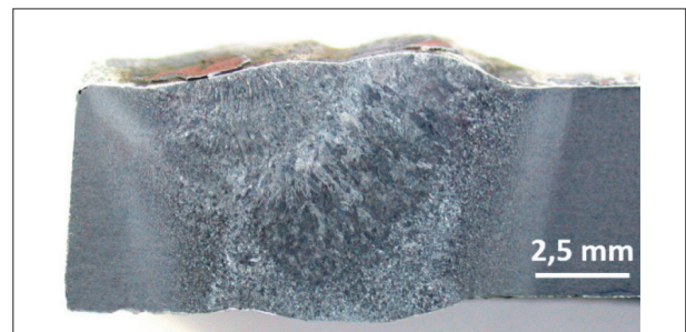
Fig. 1. Macrostructure of the T24 steel welded joint
