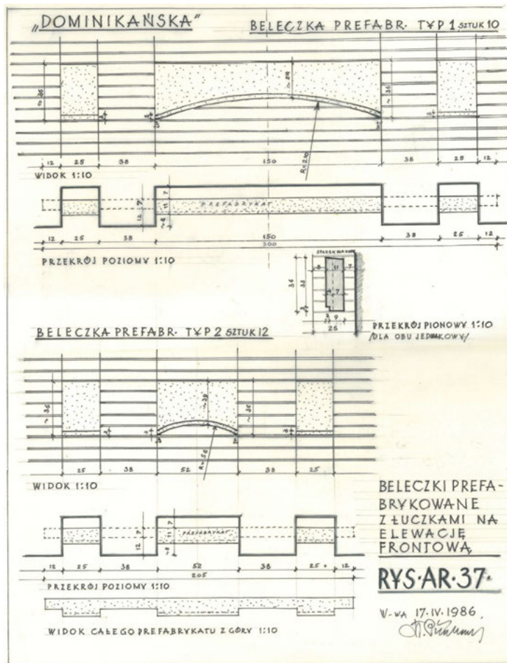
Fig. 8. Prefabricated beams with arches for the front elevation, Church of St. Dominic in Warsaw-Służew, technical drawing from the archives of the Pieńkowski family, 1986
