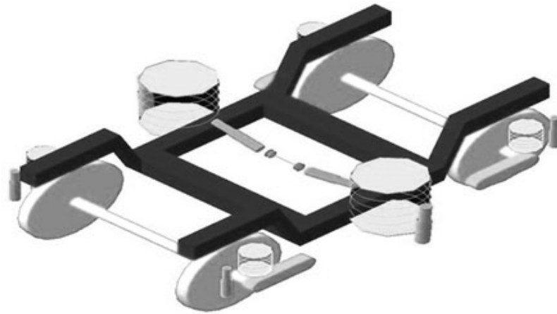
Fig. 2. Diagram of attachment of springs and dampers of a freight car cart
