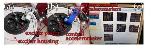
Fig. 7. Dynamic test course – mounting of piezoelectric sensors and the holder bracket on the vibration exciter: a) taking characteristics from the sample made of C35 steel,
