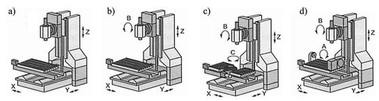
**Fig. 1.** The system of numerically controlled axes for milling machines: a) three-axis, b) four-axis, c) five-axis, d) five-axis [6]
