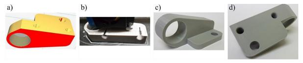
**Fig. 5.** Sample with a 20% filling made using FDM/FFF technique: a) analysis of overhanging surfaces in Ultimaker Cura 3D software, b) printout of overhangs in the threaded holes of the model, c) view of the workpiece after printing from the front, d) view of the workpiece after printing from below /own elaboration/
