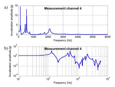
**Fig. 10.** Resonance curve for a steel cantilever measured in the direction of the dynamic excitation: a) graph on a linear scale, b) graph on a logarithmic scale /own elaboration/
