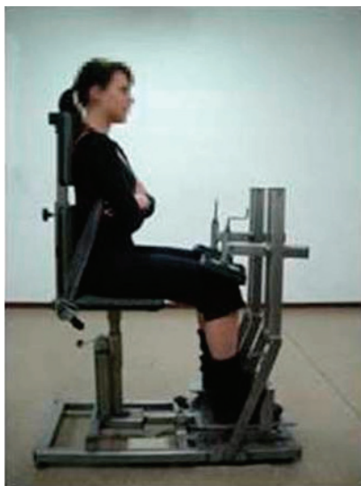
Fig. 3. A standard subject position during measurements of ankle dorsi- and plantarflexion maximal torques
