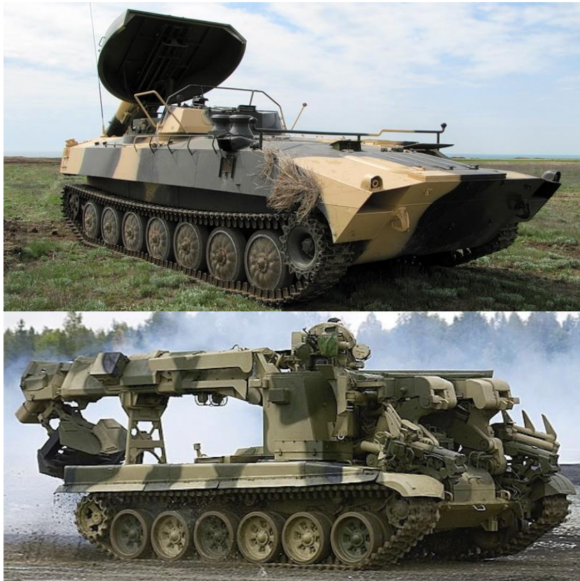
Fig. 4. Proven the UR-77 METEOR and the IMR-2/3 enable conducting passages in minefields and breaching
