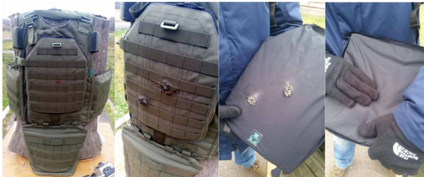
Fig. 7. Ballistic tests of the OWR-3Sz kit confirmed the resistance to 7.62 mm caliber projectile fire
