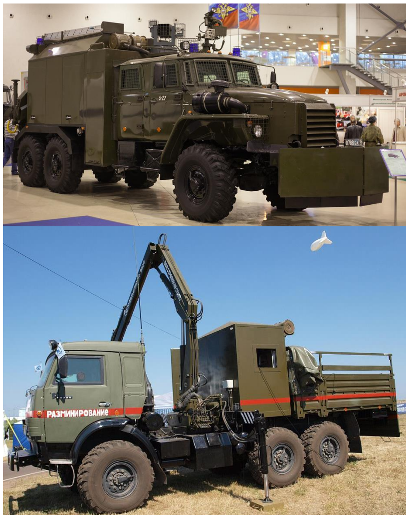
Fig. 5. The lighter Tornado based on the Ural 4320 and the Scarab based on Kamaz can be part of the RCP or light separation teams
