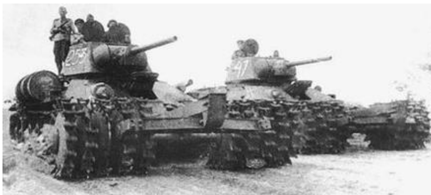
Fig. 1. The T-34 medium tank with PT-3 pressure mine flails designed by P.Murgalev
