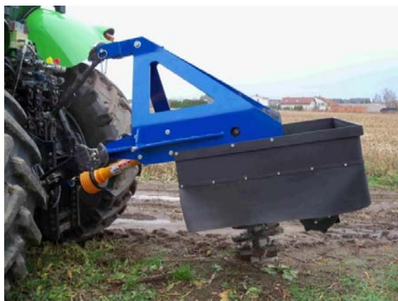
Figure 2. Model of a new machine for cutting willow rootstocks as well as bushes and young trees
