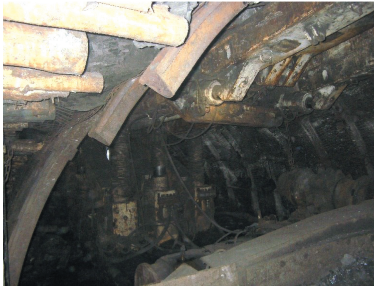
Fig. 1. Arch support door frame type ŁP with bend side wall arch
