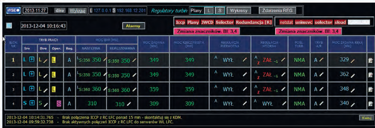
Fig. 6. The view of the LFC system main control panel
