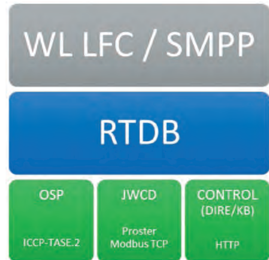
Fig. 3. Layered model of a single SRM LFC instance
