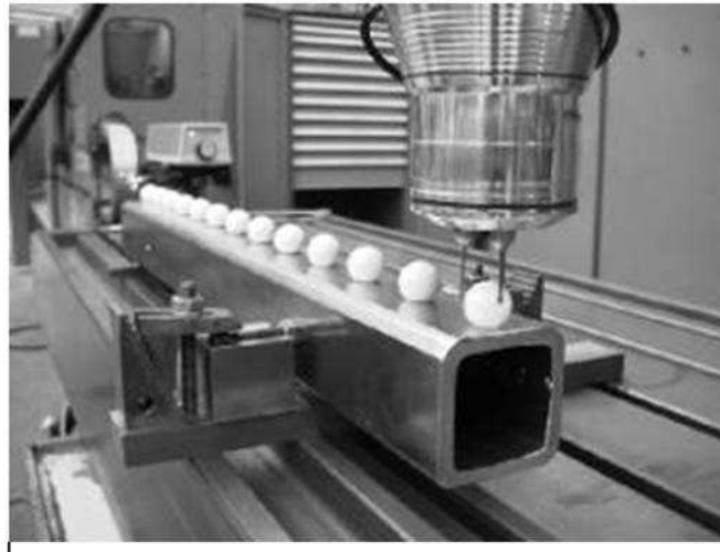
Fig. 1. Calibration using self-centering head
