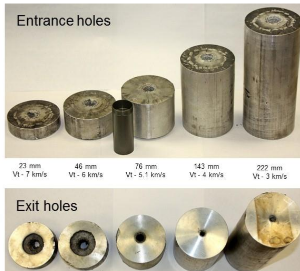
Fig. 11. Buffer plate entrance and exit holes
