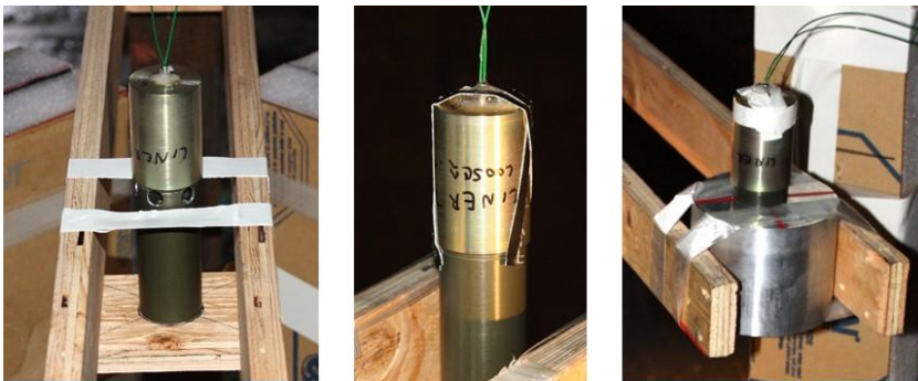
Fig. 8. Standard (c), vented (l) and larger diameter (r) buffer plate test setup
