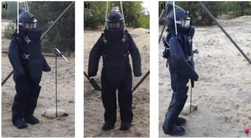
Fig. 1. Anthropomorphic test device equipped with an EOD suit, a – view with a pencil sensor, b – front view, c – view with an explosive charge
