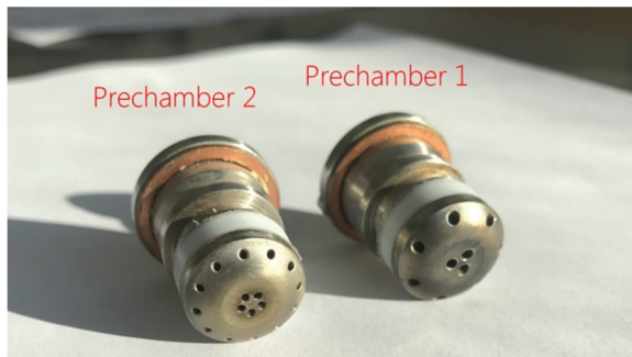
Fig. 5. Used prechambers (jet exit sides)
