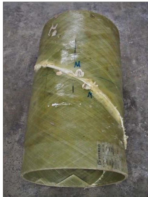
Fig. 9. Destroyed composite coating
