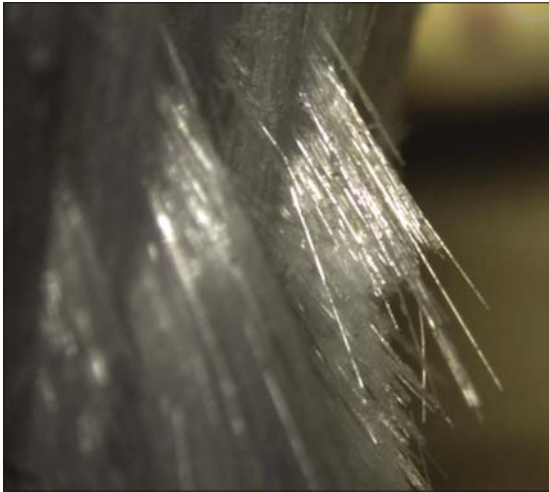
Fig. 1. Stereoscopic view of the fracture of a pipe sample made of glass fibre reinforced composite
