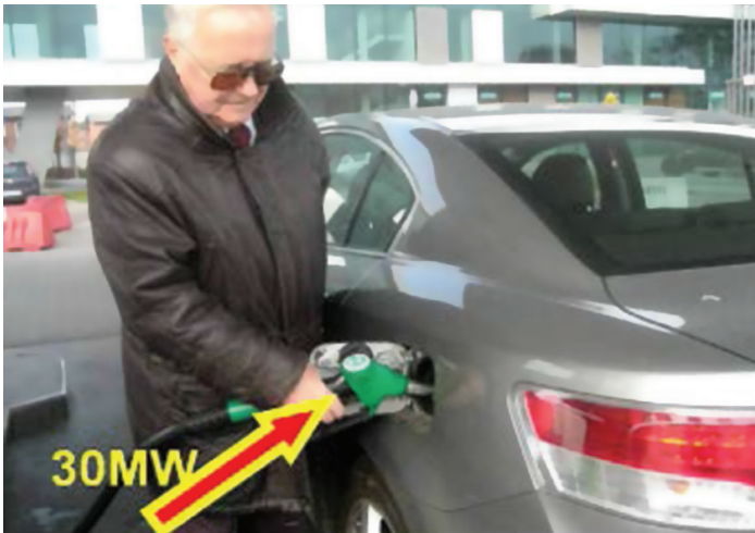
Fig. 3. Fuel power flow at refuelling
