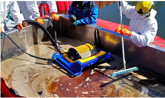
Figure 9. Assistance is needed to feed emulsified oil onto the skimmer. Photo taken during a training session in which MDO DMB was recovered with Mimimax 25 skimmer and feeding was assisted with floor squeegees. Photo: J. Halonen.
