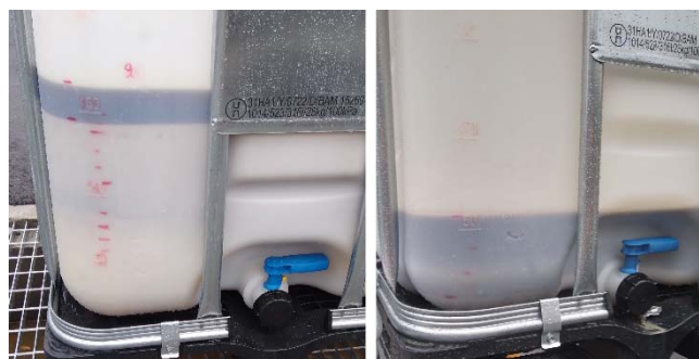
Figure 3. Recovered marine diesel oil (MDO DMB) and entrained water (free water and emulsion) separated by gravity in storage containers. On the left the recovery result of the brush skimmer and on the right the corresponding result of the disc skimmer. Photos: J. Halonen.
