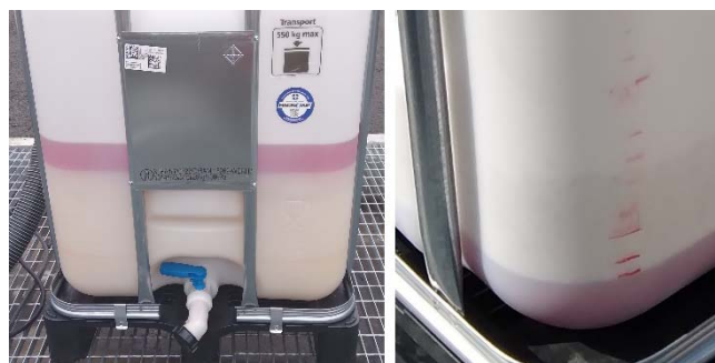
Figure 4. Recovered light fuel oil and entrained free water separated by gravity in storage containers. On the left the recovery result of the brush skimmer, on the right the corresponding result of the disc skimmer. Photos: J. Halonen.
