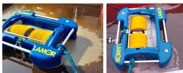
Figure 8. Emulsion formation during a brush skimmer recovery. Skimmer with a brush module recovering marine
